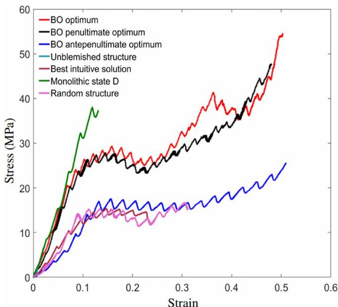
**Fig. 4. Comparison of the mechanical performance of different structures.** The stress versus strain of the BO optimum (# 1 on table S1), BO penultimate optimum (# 2), BO antepenultimate optimum (# 3), unblemished structure (# 14), best intuitive solution (# 8), monolithic state D (# 5), and representative random structure (# 11).
