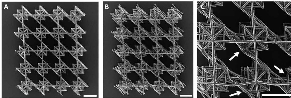
**Fig. 6. HIM images of the microlattice structure with a monolithic state D.** (A) Unloaded structure, (B) loaded structure, and (C) high magnification of part of the panel shown in (B) revealing fracture at the nodes of beam members (shown by white arrows). White scale bars, (A to C) 10  $\mu\text{m}$ .
