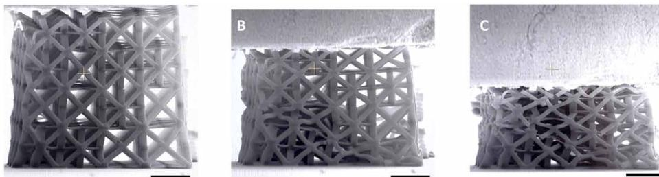
**Fig. 7. SEM images of the microlattice structure with the best intuitive solution.** (A) Before loading, (B) after loading showing excessive deformation in a sloped plane that eventually led to the collapse of the beam members on that plane, and (C) at maximum deformation showing sustained global collapse in the proximal region of the sloped plane. Black scale bars, (A to C) 10  $\mu\text{m}$ .
