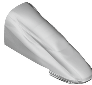
Fig. 14 The shape of the optimal train head obtained from the 3-baseline train with 2 degrees of freedom optimization
