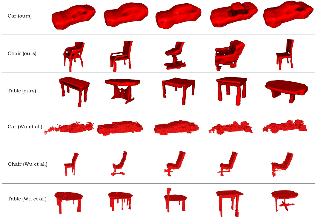
Figure 3: A sample of the shapes generated by our model using 200 dimensional random vectors sampled uniformly from U[-1, 1] . The top three rows show our generated samples and bottom three rows show samples generated by Wu et al. [1] from the corresponding classes.
