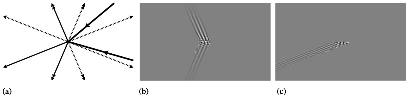
FIG. 3. Schematic and a numerical simulation of physical beams verifying the selection rules in the fourth column and top two rows of Table I. Here, \theta^{\text{in}}(0) = 40^\circ and \theta^{\text{in}}(4) = -16^\circ , so |\chi| < 1/2 . (a) (left) Schematic shows: two incoming primary beams from the right as heavy arrows; the three allowable (according to Table I) outgoing harmonics as thin solid arrows; and the five disallowed harmonics as dotted arrows. The high frequency harmonic St. Andrew's cross has two arrowheads and the low frequency harmonic has one. (b) (center) The vorticity in a numerical simulation with output filtered to show only frequencies with \omega^{\text{out}} = \pm(|\omega^{\text{in}}(0)| + |\omega^{\text{in}}(4)|) , i.e., the high frequency harmonic or top row of Table I. (c) (right) As in (b), but filtered to show frequencies \omega^{\text{out}} = \pm(|\omega^{\text{in}}(0)| - |\omega^{\text{in}}(4)|) , i.e., the low frequency harmonic or second row of Table I.
